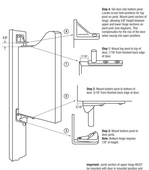
with jamb hinge section over pivot post.
